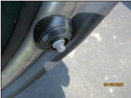
(Missing bolt cover caps beneath seat)
